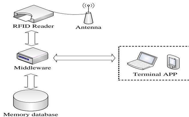
**Figure 2.** The basic structure of the RFID system
