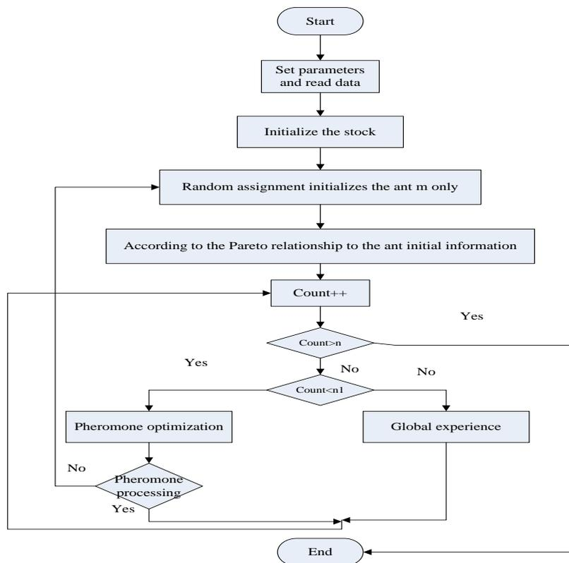
Figure 1. Total flow chart of ant colony algorithm
