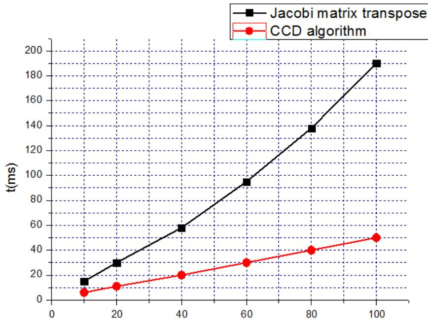
**Figure 4.** Comparison of convergence of Jacobi matrix transpose method and CCD algorithm
