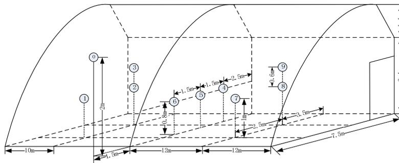
Figure 2. Solar greenhouse structure diagram
